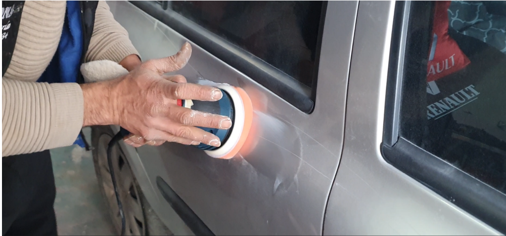
Figure 2.2: We visited a car repair shop to learn more about "scratch removal" by polishing. We observed that the expert applied the right amount of pressure to the surface in the normal direction while following a circular trajectory in the tangential direction to remove a scratch.
