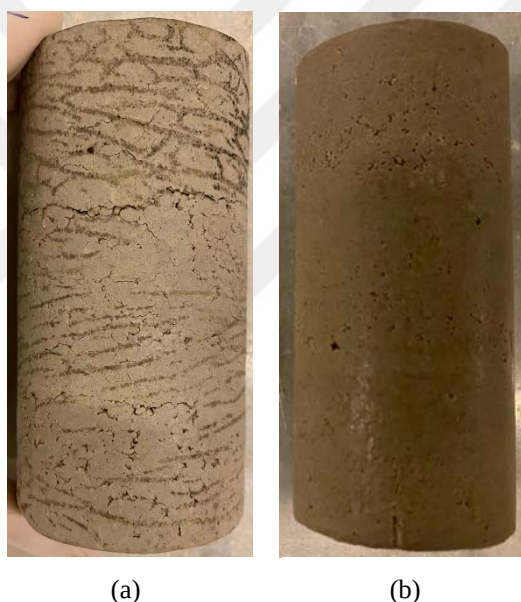
Figure 4.27 : Untreated (a) and 14% \text{MgCl}_2 -treated (b) soil samples before the 7 th freeze-thaw cycle.
