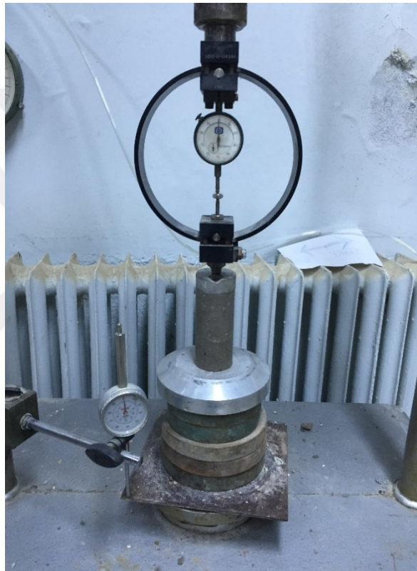
Figure 3.6 : Unconfined compression device.
