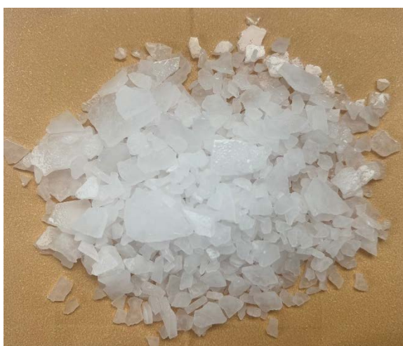
Figure 3.11 : The appearance of 3.2.3 magnesium chloride hexahydrate ( \text{MgCl}_2 \cdot 6\text{H}_2\text{O} ) flakes.
