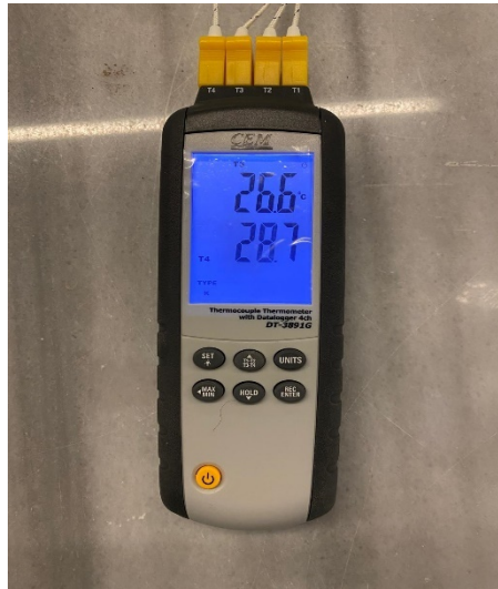
Figure 3.4 : Thermometer device used for freezing point measurements.
