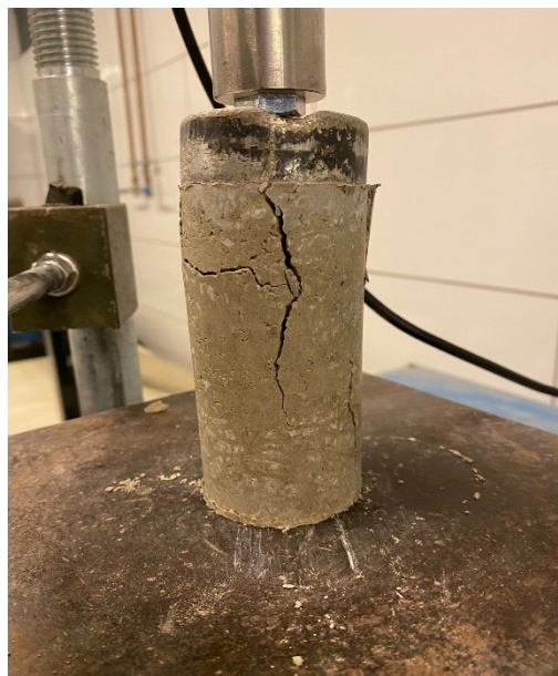
Figure 4.8 : PEG-cement-treated clay sample with 7% cement and 20% PEG.
