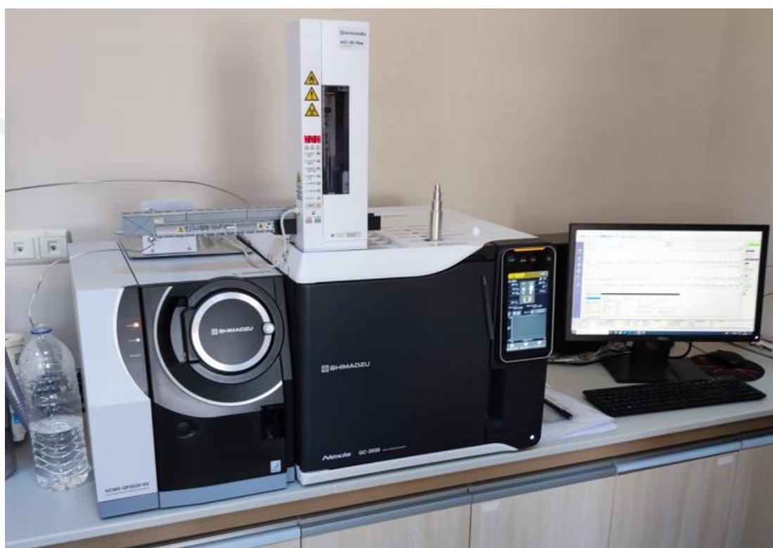
Figure 3.10. Shimadzu GC and GC-MS system for volatile analysis
