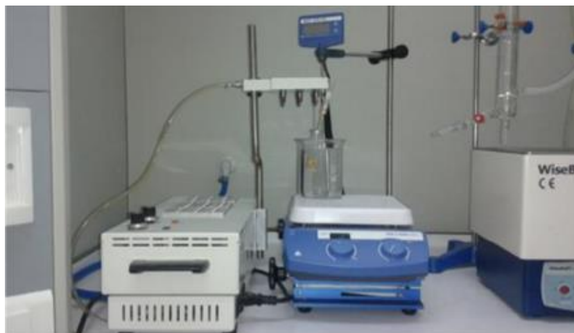
Figure 3.8. Purge and Trap System for aroma compounds extraction
