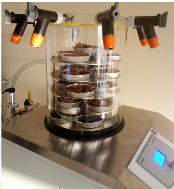
Figure 3.6. Freeze drying process of fermented cocoa beans applied in this study
