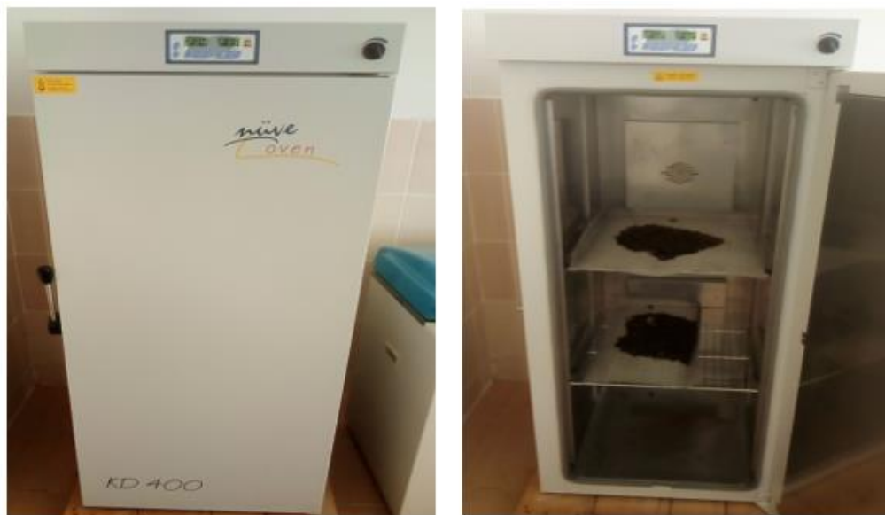
Figure 3.4. Hot air convective drying process of fermented cocoa beans used in this study
