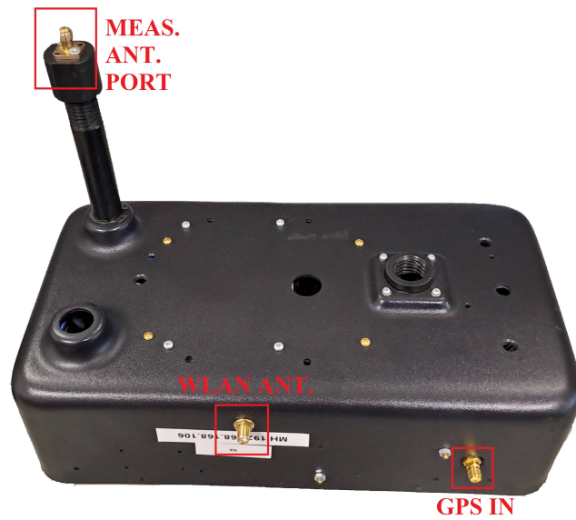
Figure 2.10 : Channel measurement system – Enclosure and antenna ports.
