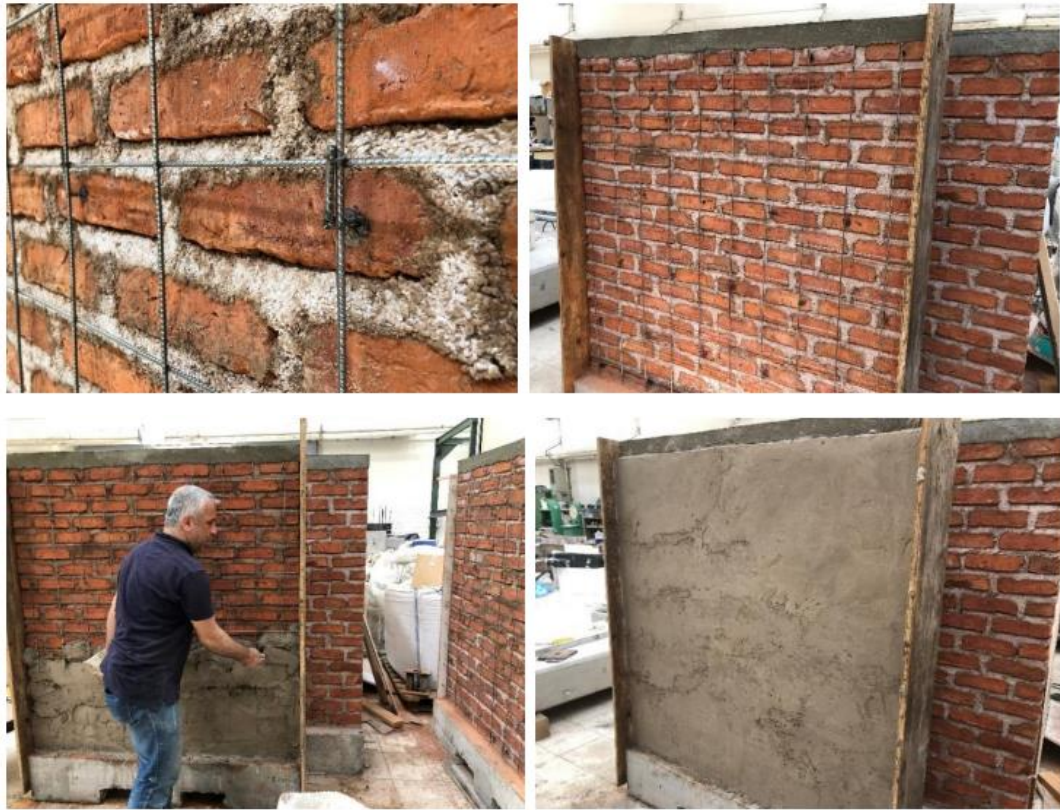
Figure 2.8. Steel mesh and 4 cm thick Khorasan mortar application [16].
