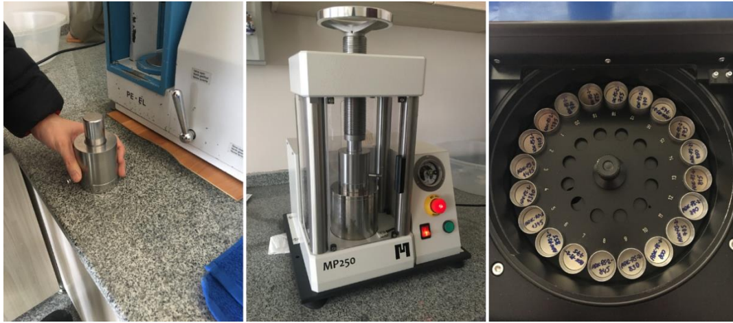
Figure 4.4. Pellet preparation procedure for XRF analyses
