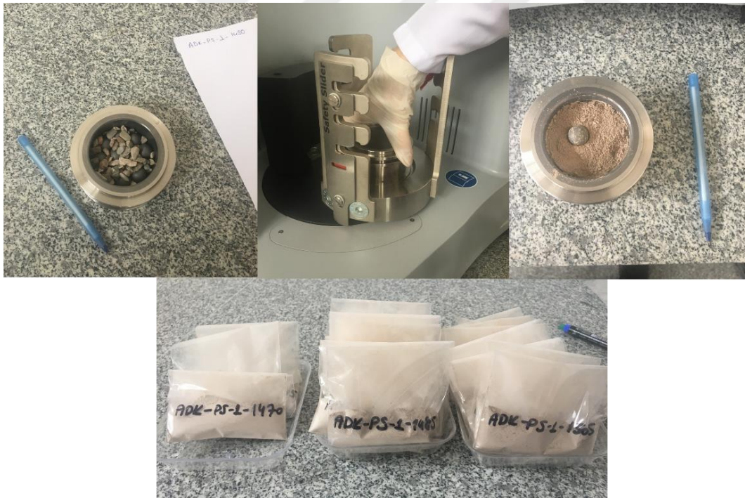
Figure 4.2. Fine grinding procedure for XRD and XRF analyses
