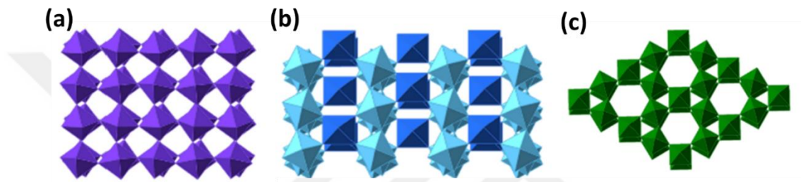
Figure 4.3 : (a) Monoclinic, (b) orthorhombic and (c) hexagonal crystalline phases of WO 3 .
