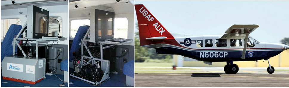
Figure 12: ARCHER hyperspectral remote sensing system installed on GippsAero GA8 [30].
