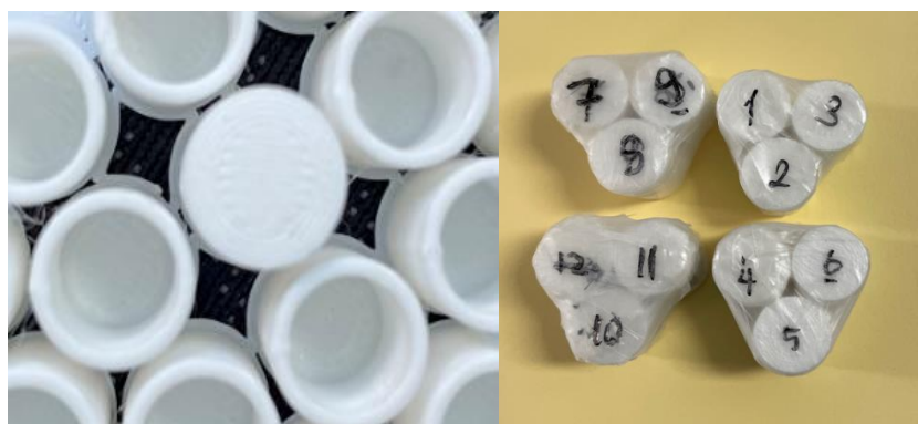
Figure 3.5 Photographs of sample holder printed by 3D printer
