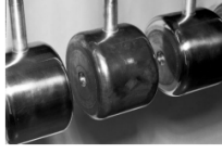
CERN LINAC 2 tank 1: 200 MHz 7 m x 3 tanks, 1 m diameter, final energy 50 MeV.
