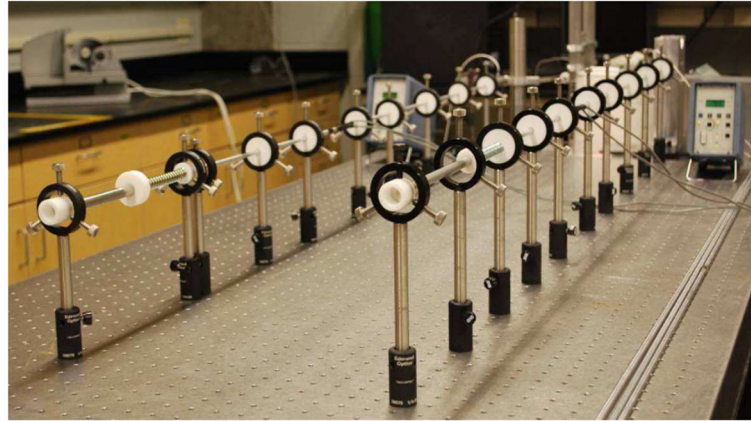
Figure 16: Miniaturized split – Hopkinson tension bars [18].
