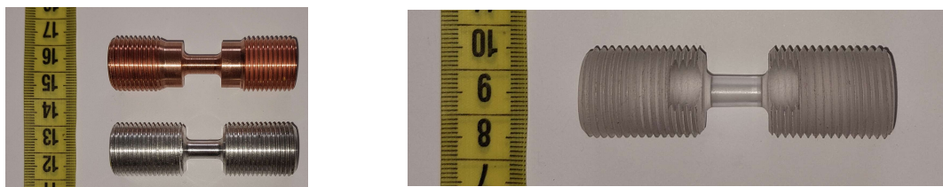
Figure 35: OFHC Copper, AA6061-T6 and Polycarbonate specimens.
