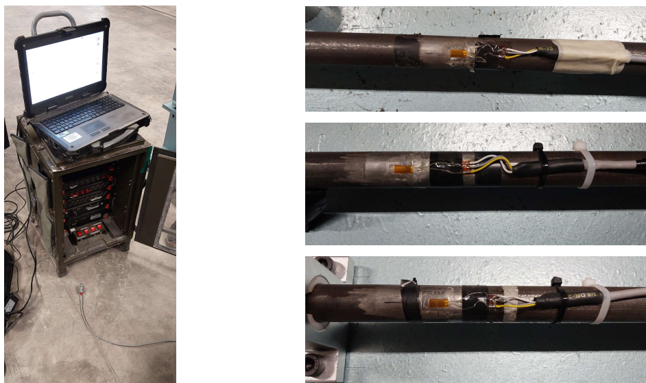
Figure 30: Strain gauges and Dewesoft data acquisition system
