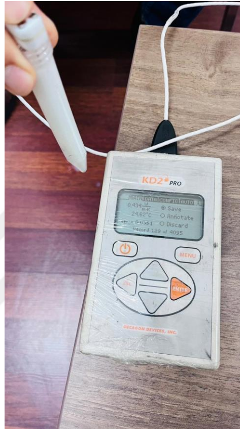
Figure 4.6 A view of measurements made with KD-2 Pro thermal conductivity measurement device
