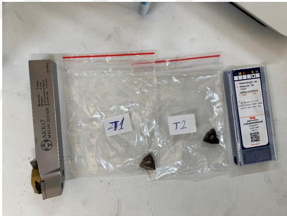
Figure 4.9 A photograph of cutting insert and cutting tool holder used in the machining experiments
