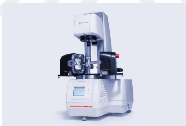
Figure 4.5 The photograph of Anton Paar brand MCR 702-e compact rheometer [55]
