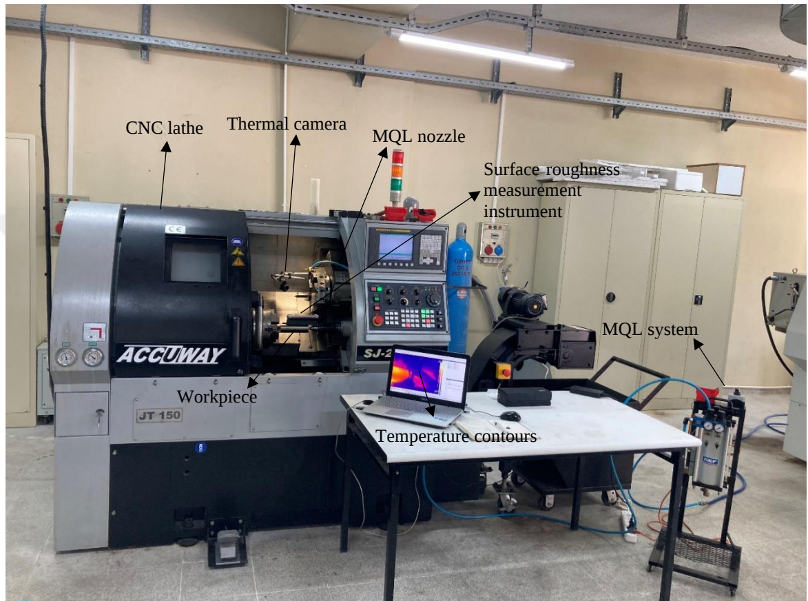
Figure 4.7 A photograph of the experimental setup for the machining
