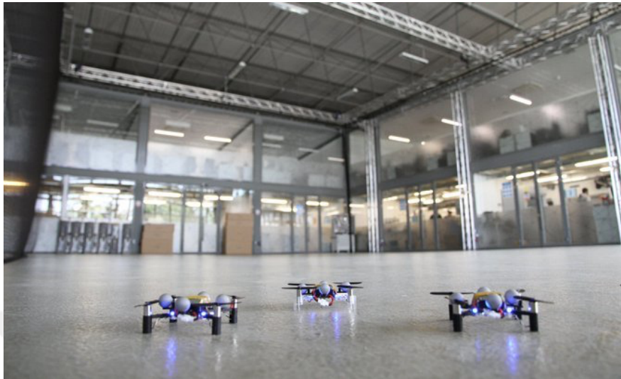
Figure 3.3 : Test Environment with 8 motion capture cameras (VICON V16) and 3 nano-size drones (Crazyflie)
