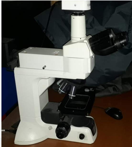
Figure 3.5. Nikon Eclipse LV150 Optical Microscope with Clemex Imaging Apparatus Additionally, Scanning Electron Microscopy (SEM) was utilized to analyze the formations that appeared by etching the alloy. Energy Dispersive X-ray Spectroscopy (EDS) was also used for the identification of the oxides.
