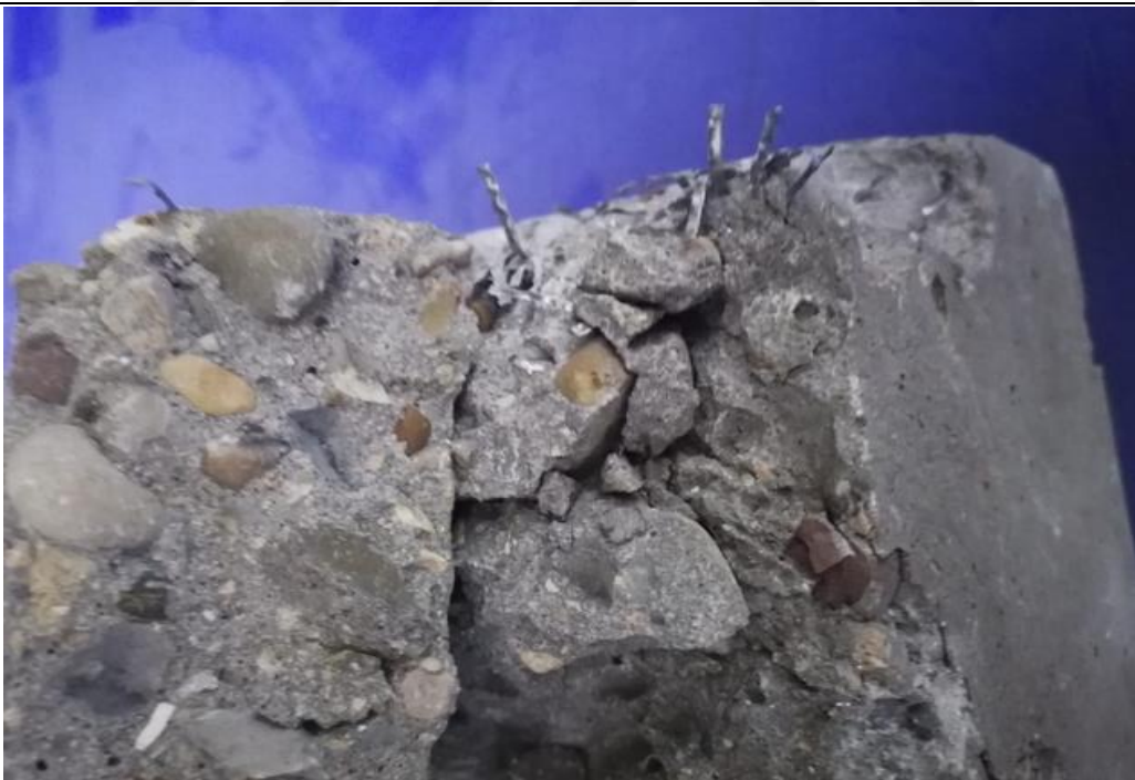
Figure 4.1: Cubes After Compression
