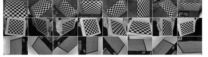
Fig. 6. Arbitrary shots for each of the three calibrators: 1m^2 checkerboard (top), A4 sized checkerboard (center), and catenary (bottom).
