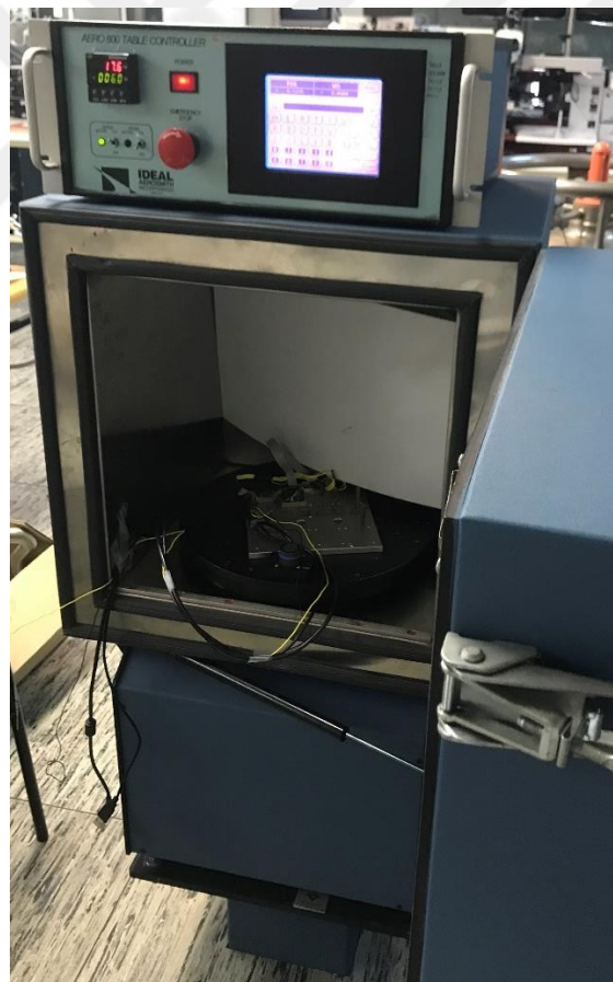
Figure 5.21. Temperature characterization setup for different amplitude ratios of the FM gyroscope
