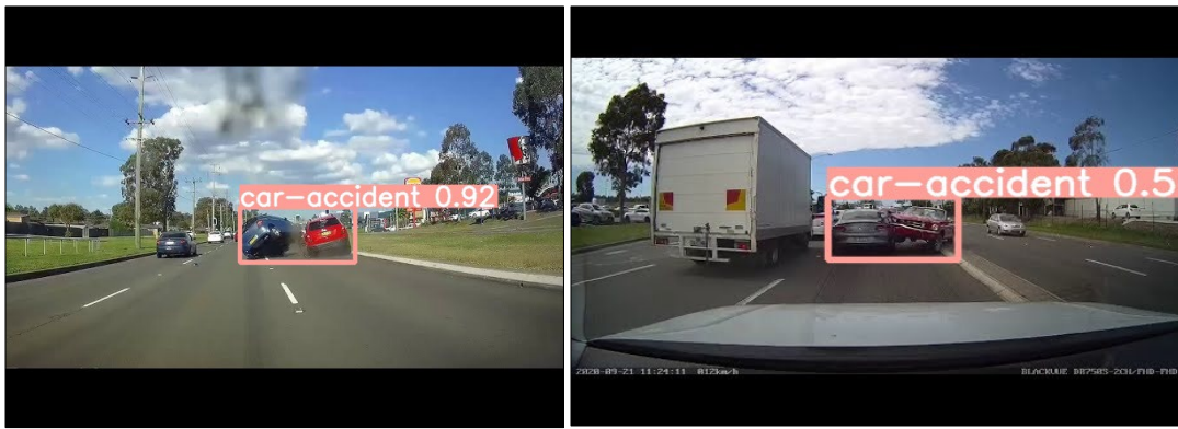
Figure 4.4 Accident Detected by YOLOv5 Itself
