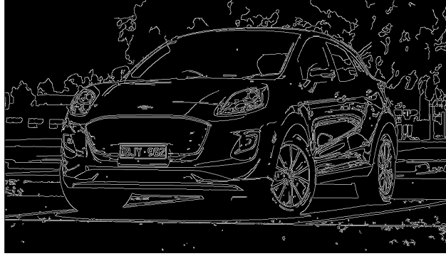
Figure 3.28 The Effect of Bilateral Filter and Canny Edge Detection (step 2)
