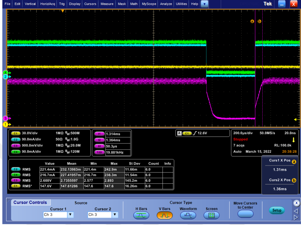
Figure 54 Dimming slew rate adjustment for current compensation
