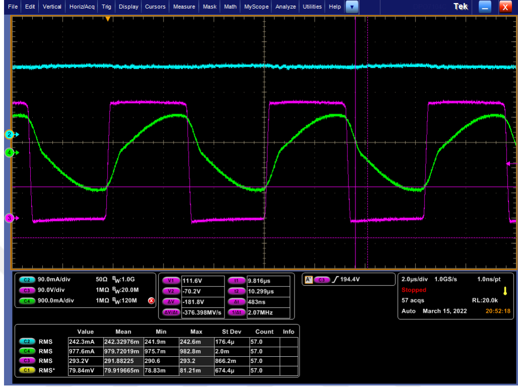
Figure 53 String_2 LED current, primary resonant current and gate signal of MOSFET_1
