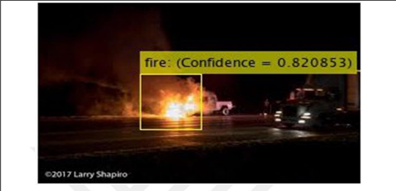
Figure 4.3: shows the fire detection mechanism.
