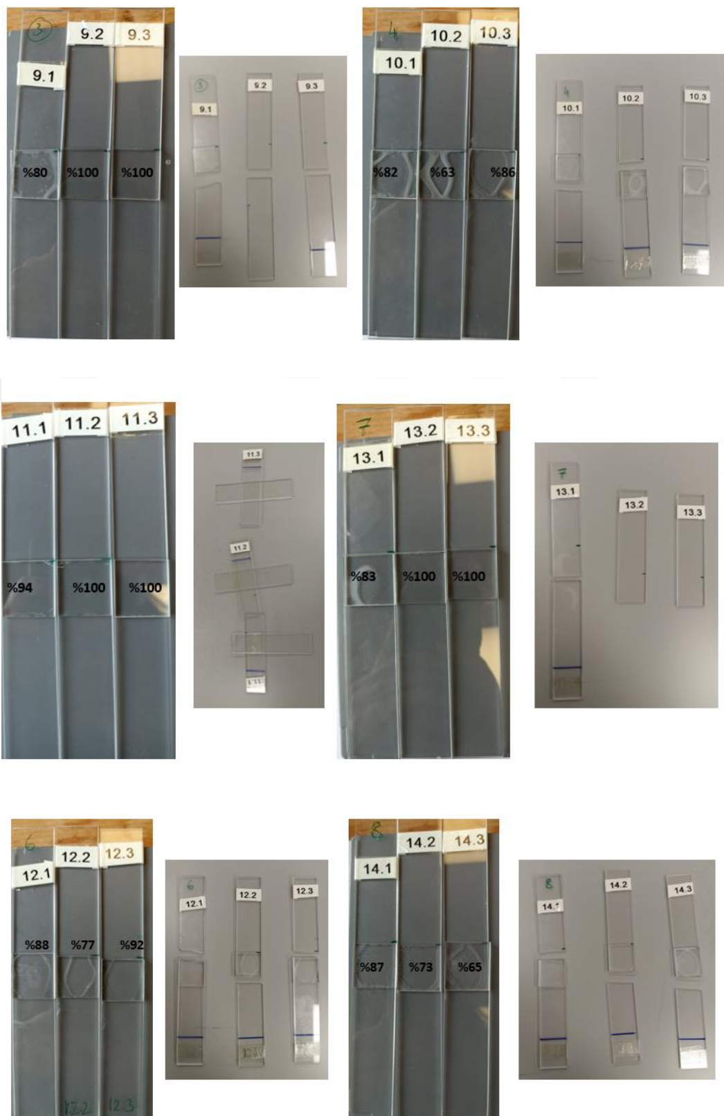
Figure 3.10: Pictures of bonded PMMA (25x25mm) before and after bonding strength experiments with room temperature.
