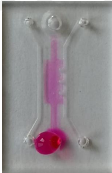
Figure 2.15: Image of h=150/400 \mu\text{m} channel heights of three grooves having 600 \mu\text{m} diameter loading with Rhodamine B dye-stained water.
