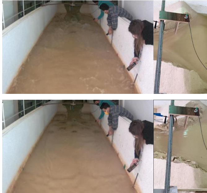
Figure A.B.1: Camera 2 (flow and sediment transport at downstream area) and Camera 1 (stages of breach formation) at a) 249 sec, b) 300 sec, c) 305 sec, d) 316 sec, e) 354 sec, f) 384 sec for experiment OR2
