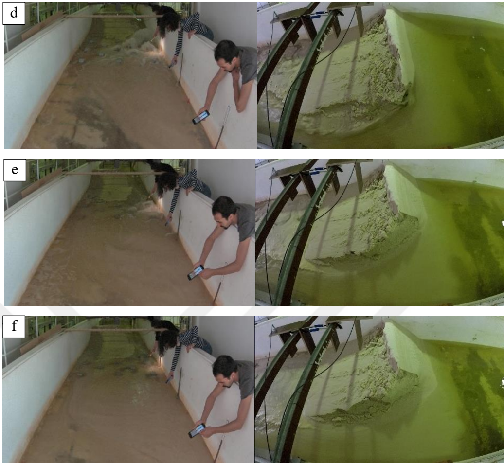
Figure 4.23: Camera 2 (flow and sediment transport at downstream area) and Camera 1 (stages of breach formation) at a) 175, b) 310, c) 325, d) 340, e) 390, f) 435 for experiment PR1
