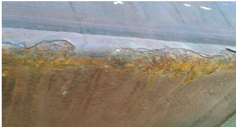
Figure 2.4 Bonnet of a ship (guide to inter-granular corrosion).
