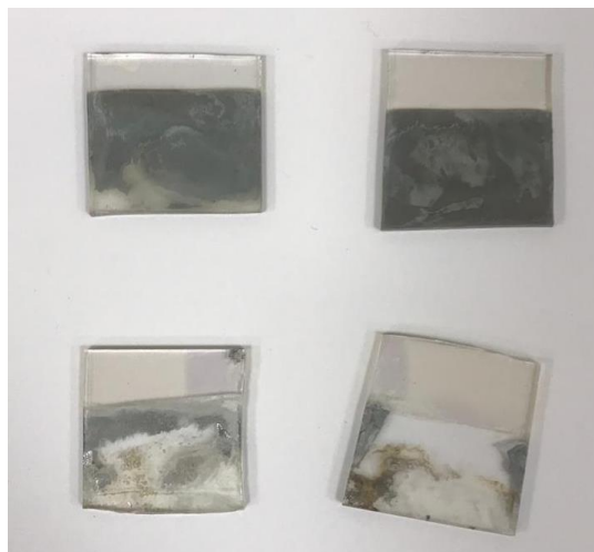
Figure 5.2: Coatings under different voltages.
