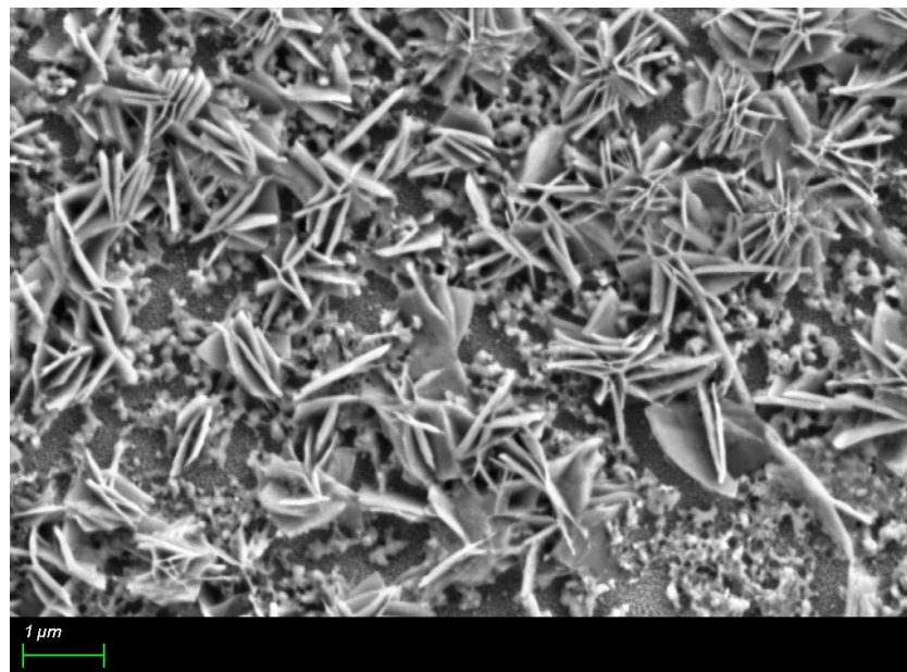
Figure 5.7: SEM image of ZnO nanostructures on glass/ITO/Zn substrates.
