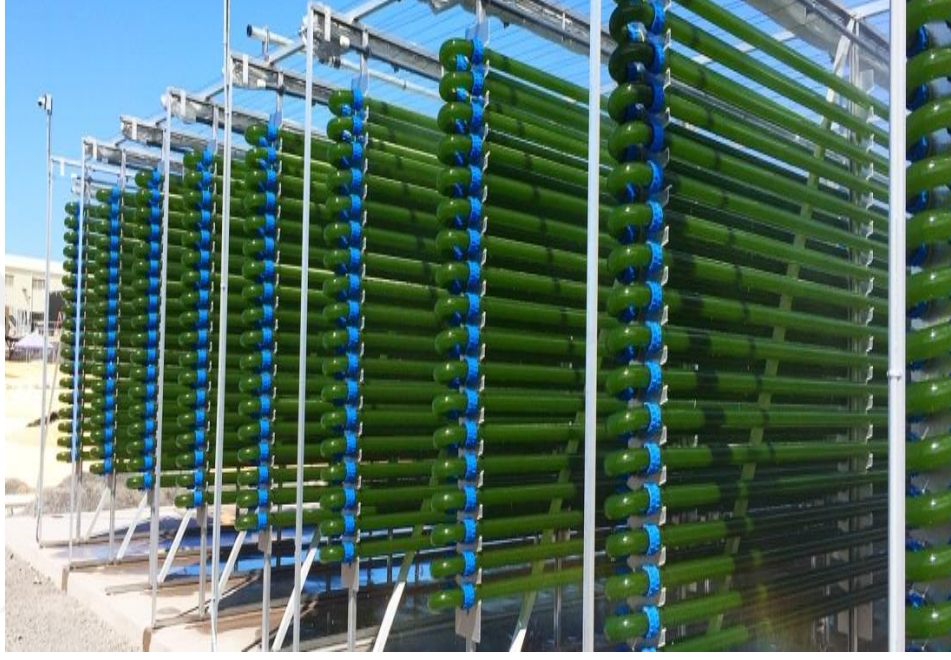
Şekil 2.2. Tübüler alg sistemi ( http://www.varicon aqua.com/products-services/phyco-flow/ ).
