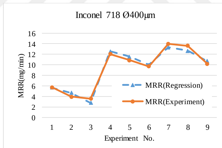
Figure 5.37 Comparison of mathematical model and experiment results of MRR for Inconel 718, Ø400µm
