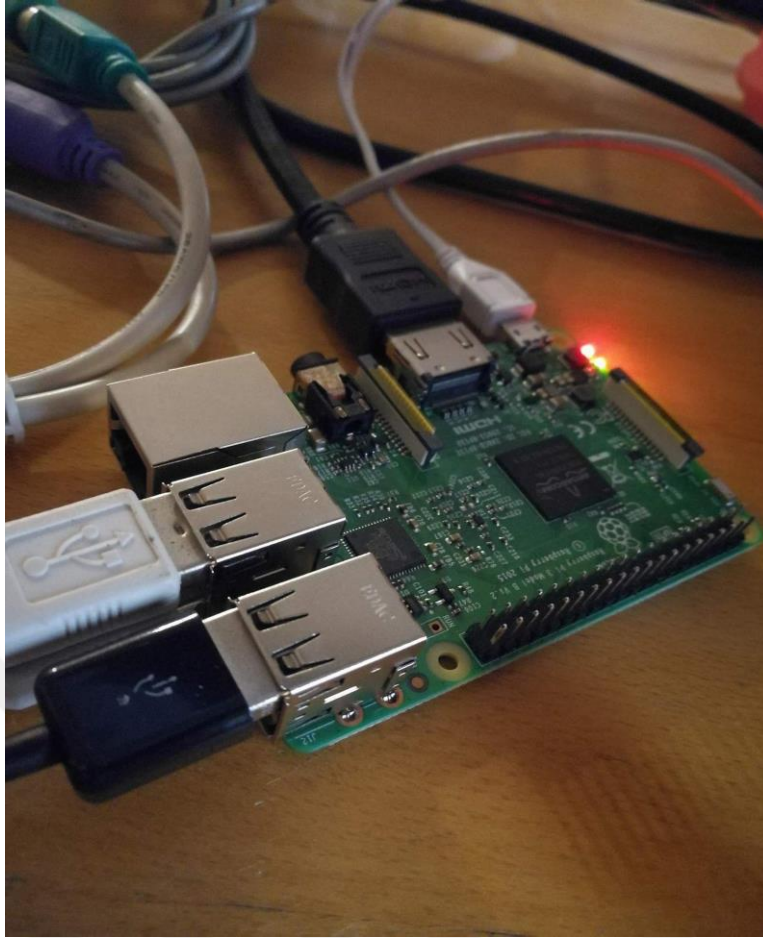
Figure A.6 RaspberryPI as a gateway (Karaduman et al., 2018a, 2018b)
