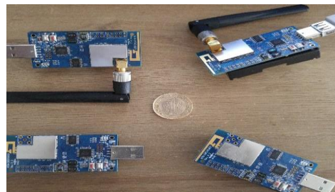
Figure 4.1 The sink and source nodes.
