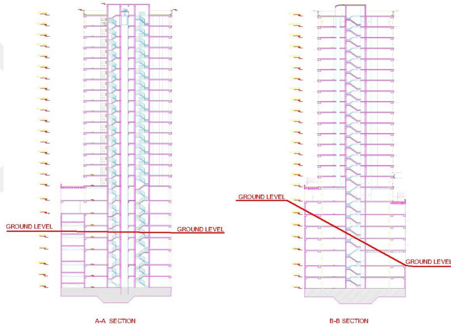
Figure 2.5 : The ground levels of the building.
