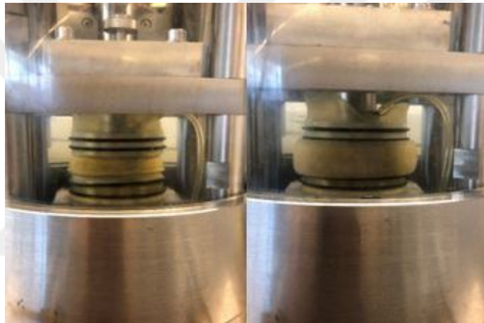
Figure 4.6 : Samples that collapsed during the experiment with the recommended K_0=1.0 setting.
