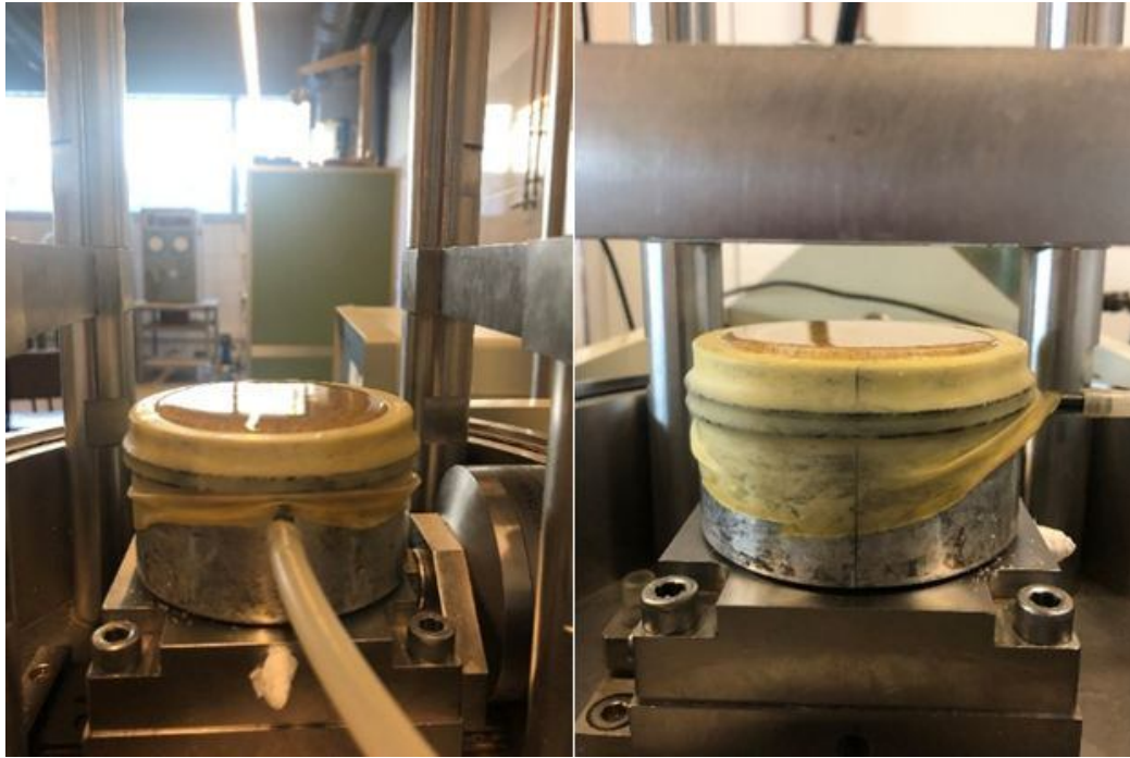
Figure 3.8 : 24 hours after the prepared partially saturated sand sample.
