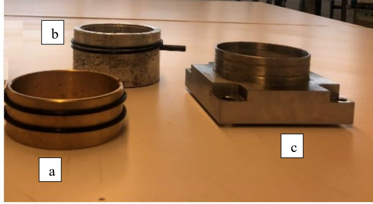
Figure 3.4 : (a)O-ring tool, (b) split mold and (c)base pedestal of the test device.
