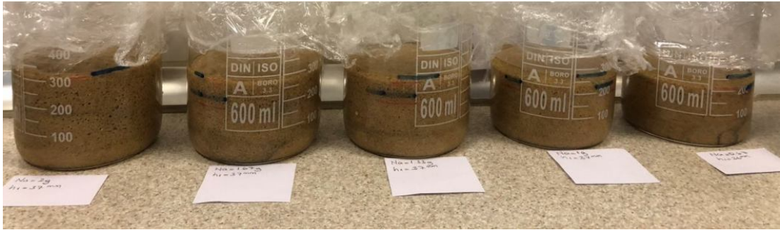
Figure 3.7 : Specimens prepared to obtain degrees of saturation in terms of different ratios R .
