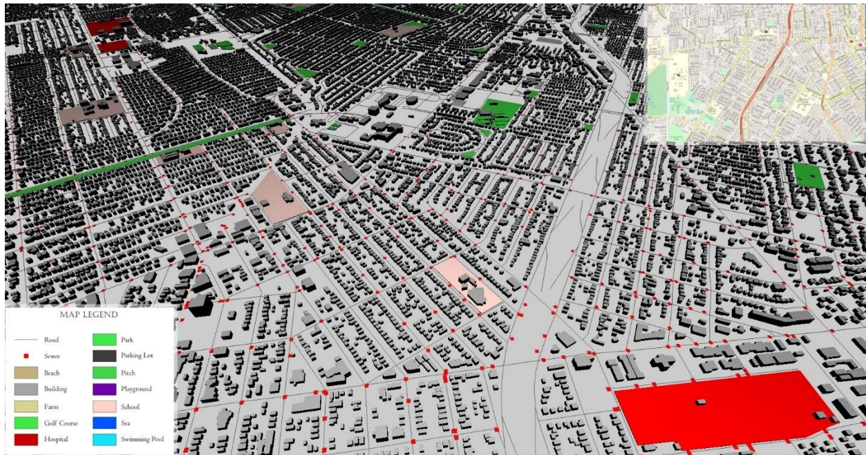
Figure 50. Visualization of storm drains in Corpus Christi
