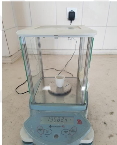
Calculate the weight of the crucibles and specimens
