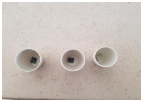
Specimens (MWCNTs-COOH, MWCNTs and PET respectively) before positioned in furnace
