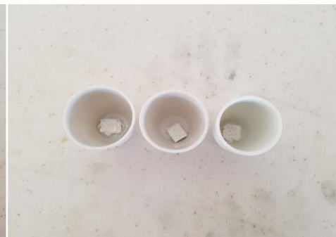
Specimens after positioned in furnace (pure reinforcement results)
