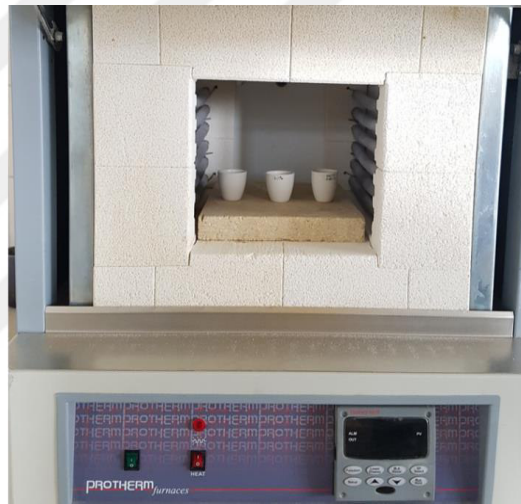
Specimens in the furnace and the temperature set to 620 °C
