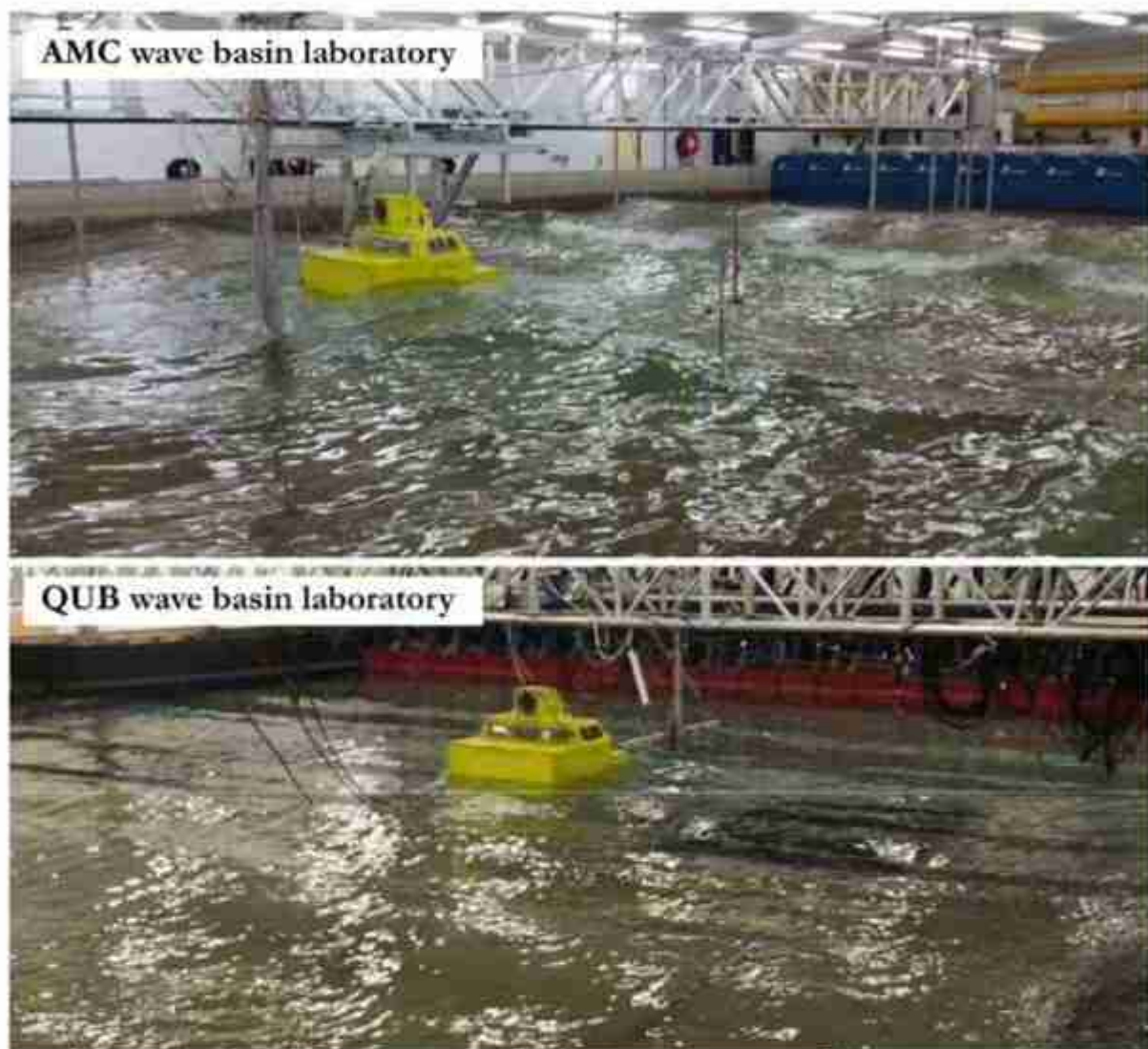
Figure 2-6: Experimental Setup for same WEC Device in AMC and QUB Laboratories, Orphin et al.(2022)
