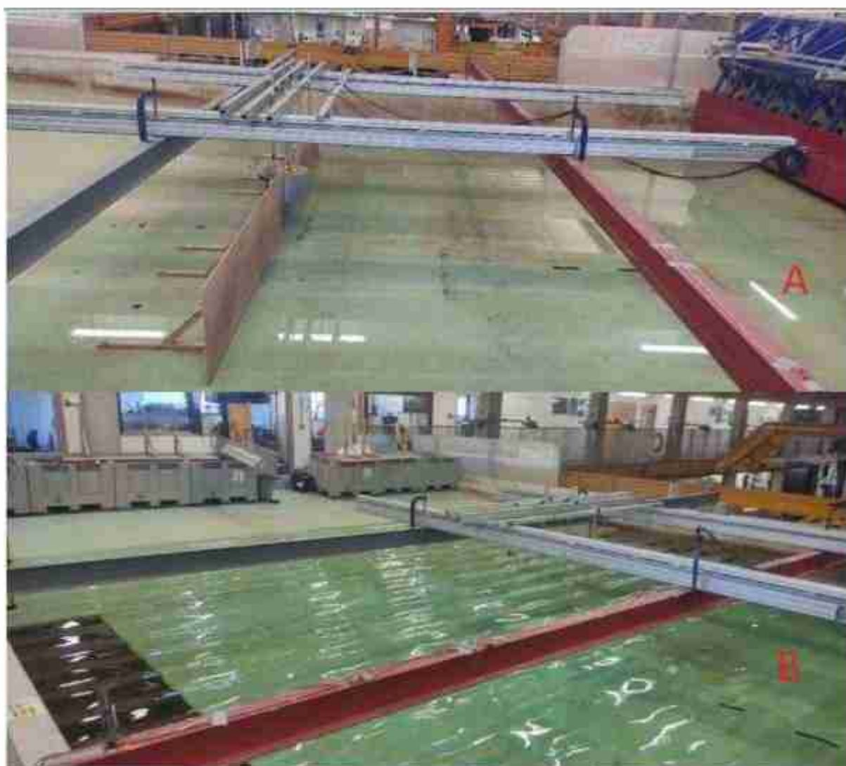
Figure 3-1: General View of Experimental Setup With Breakwater (A), and Empty Basin Test Setup (B)
