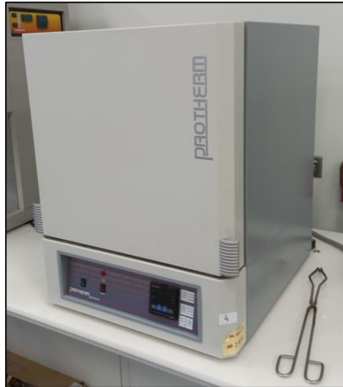
Figure 2. 5. Furnace setup for the thermal oxidation in air atmosphere.
