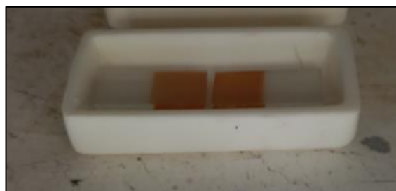
Figure 2. 3. The hematite achieved samples after the oxidation procedure.
