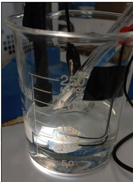
Figure 2. 8. Photoelectrochemical measurement setup with the 3 electrode system, using a solar simulator for the illumination.
