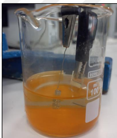
Figure 2. 1. Thin Fe coating with using electrodeposition in a electrode system with two-electrodes on the FTO substrate
