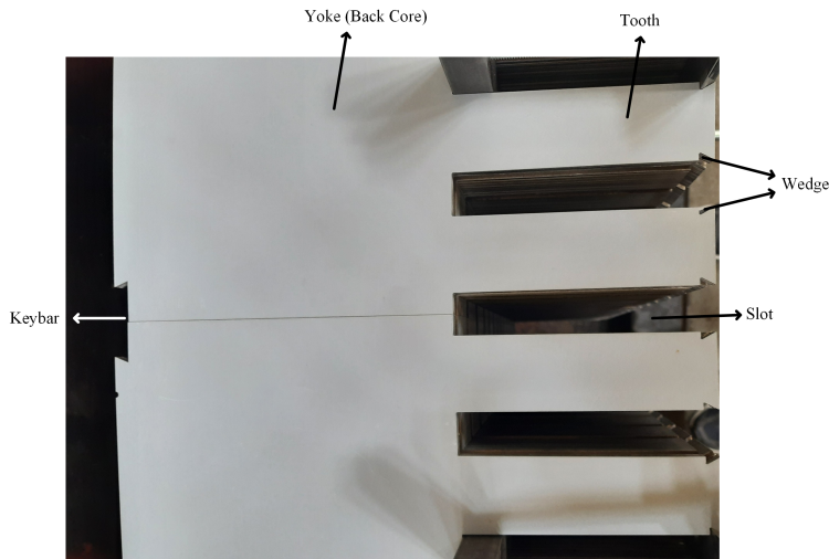
Figure 2.8: Stator core lamination.
