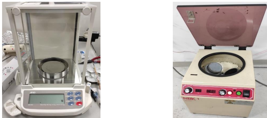
Figure 2.6 On the left the balance and on the right the ball mill mixer
