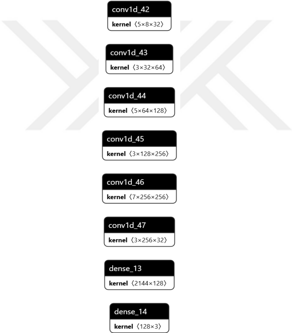
Figure 2.5: Proposed CNN Architecture layer specific details.
