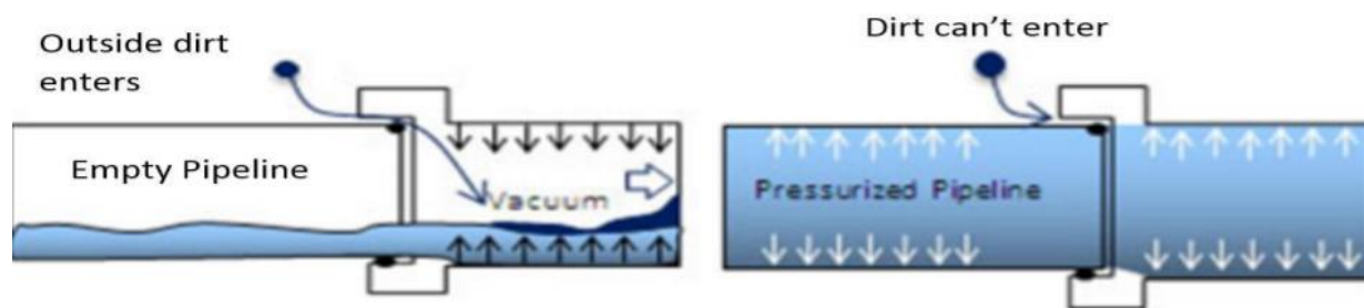
Figure 3: The case of an empty pipeline and a pressurized pipeline (Farmani, 2018)
