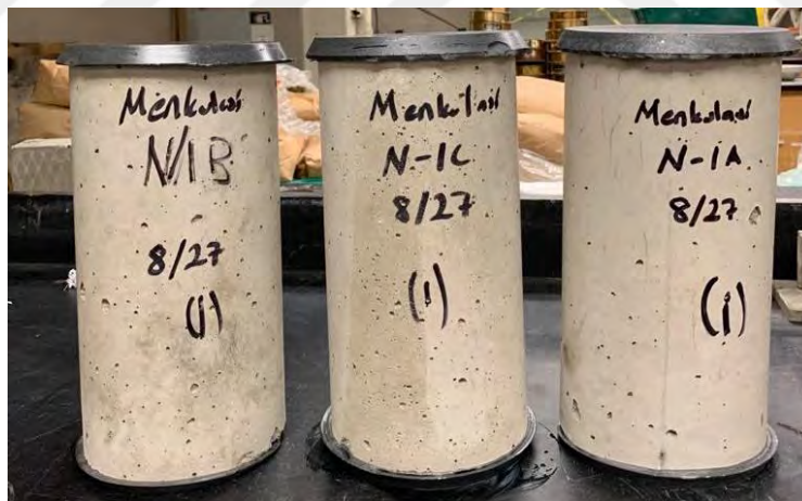
Figure 3.24. Sulfur capped concrete samples for creep and shrinkage tests
