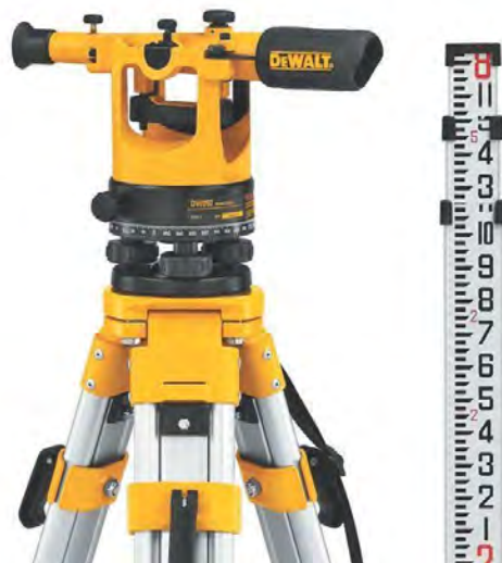
Figure 2.2. Differential level instrument, tripod and surveying rod
