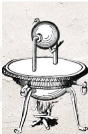
Figure 2.4 : Heron's Gas Turbine [3].
