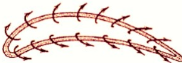
Figure 4.8 : Transpiration Cooling Figure [14].
