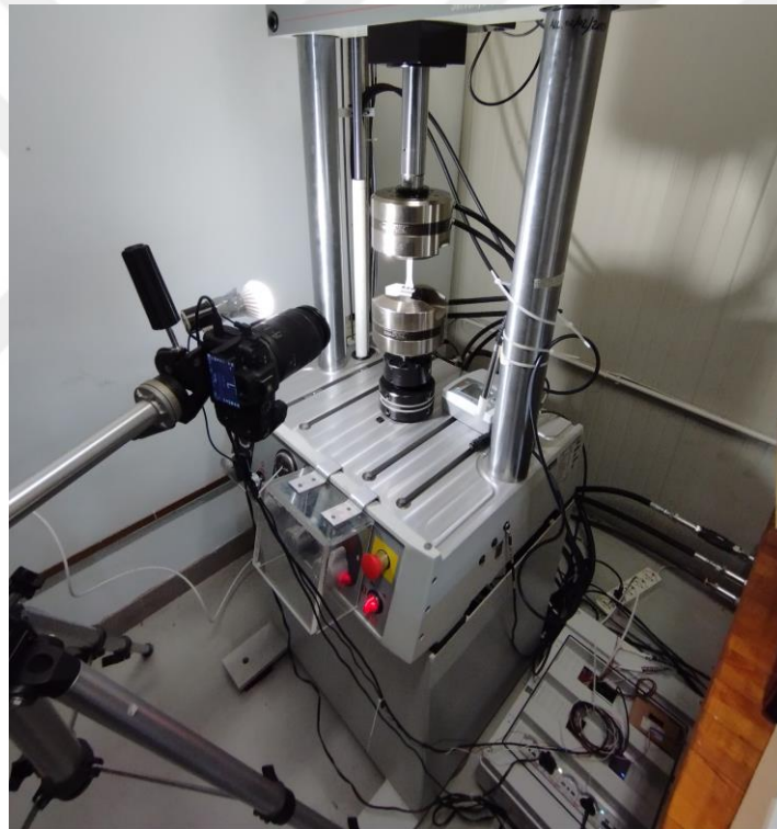
Figure 2-6: Fatigue testing setup
