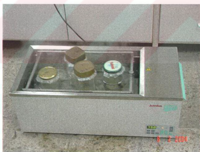
Figure 8.2. Shaking water bath used in the experiments
