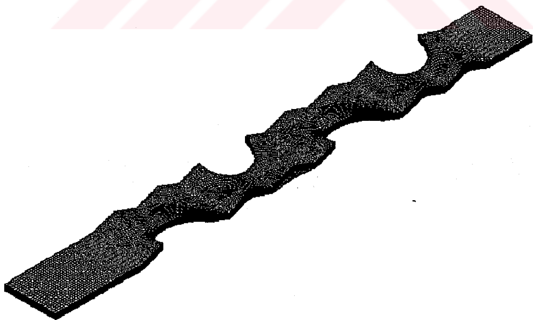
Figure 4.13. Global mesh of the computational domain for the four cylinder of staggered layout and wavy fin configuration
