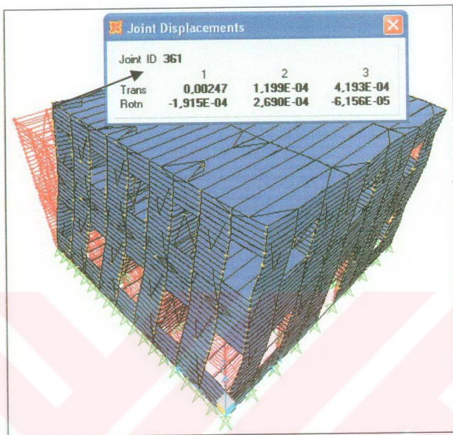
Figure 5.18 Deformed Shaped of Bağdadi Type Building With Infill
