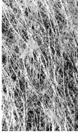
Figure 2.4 Typical Chopped Strand [5]
