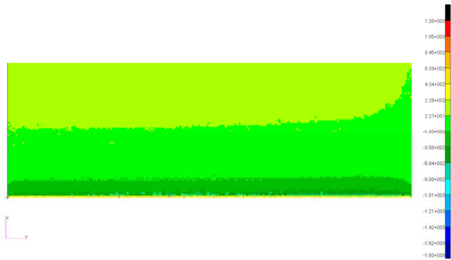
Figure 4.13 Cruise Condition Pressure Load Contours for Lower Skin, Aerodynamic Mesh [Pa]
