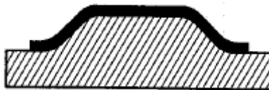
Figure 2.8 Example for Male Tool [4]
