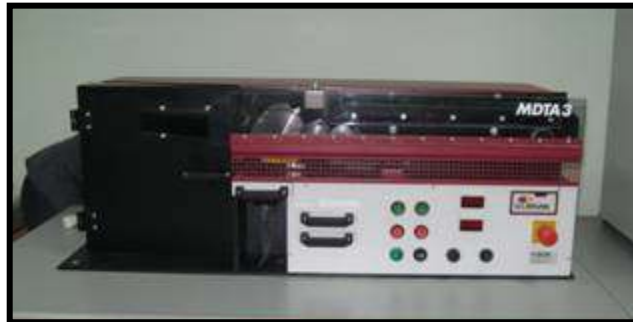
Şekil 5.16. MDTA 3 (Micro Dust and Trash Analyzer).
