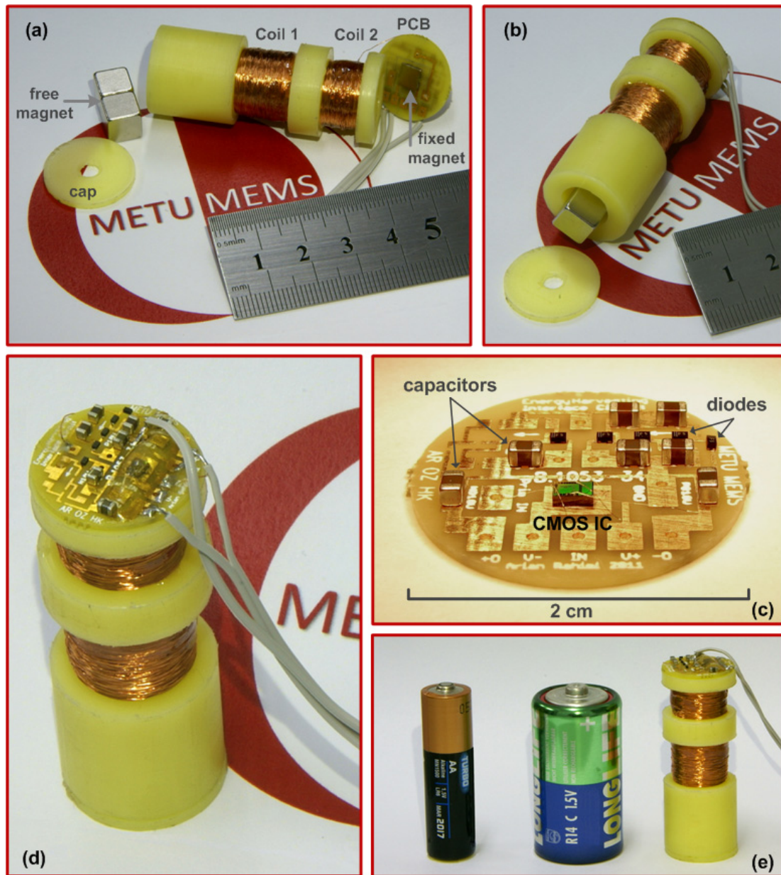
Figure 5.31: Photographs of the proposed energy harvesting system. (a) fixed magnet attached to the backside of the PCB, (b) the free magnet placed to the cylindrical tube, (c) photograph of the PCB indicating the utilized diodes, capacitors, and the CMOS IC, (d) completely assembled system, and (e) size comparison with AA and C-type batteries.
