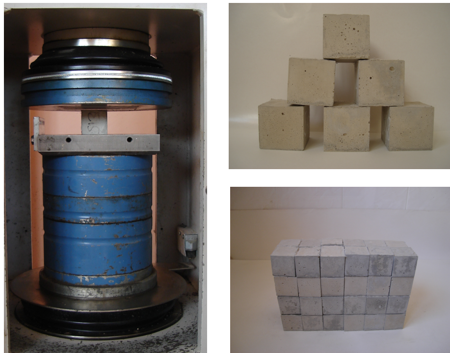
Figure 3.9 Compression testing machine and cubic samples
