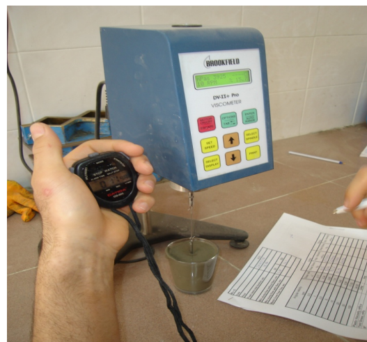
Figure 3.8 Rotational viscometer test
