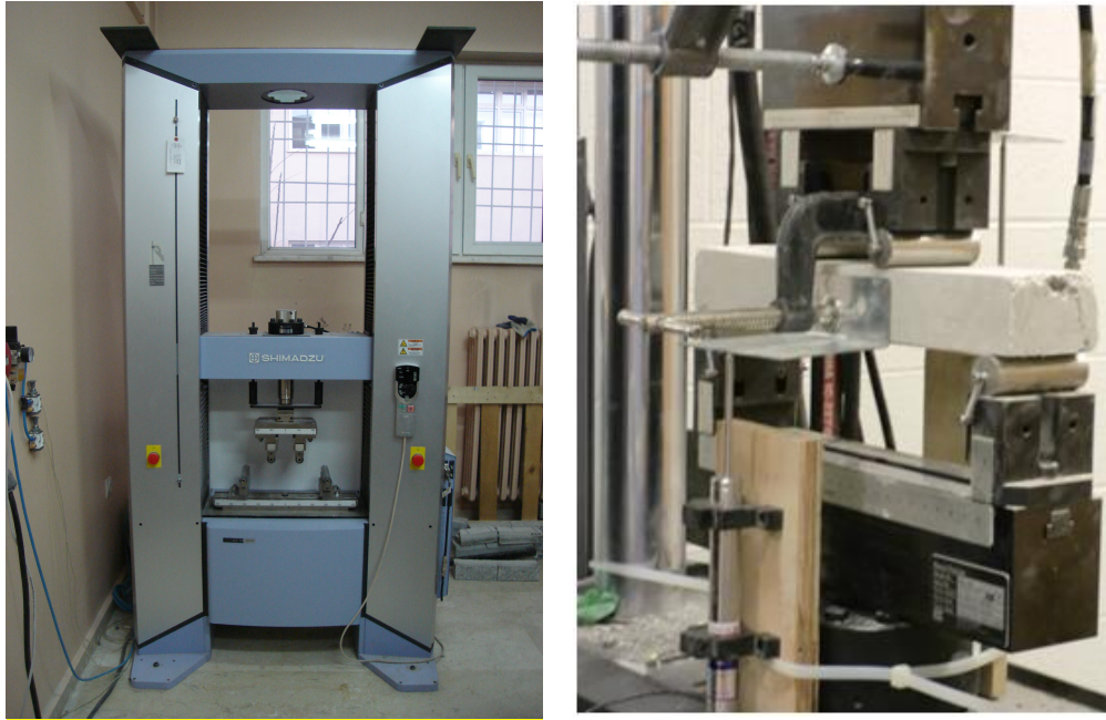
Figure 3.11. Four-point Flexural Strength test machines
