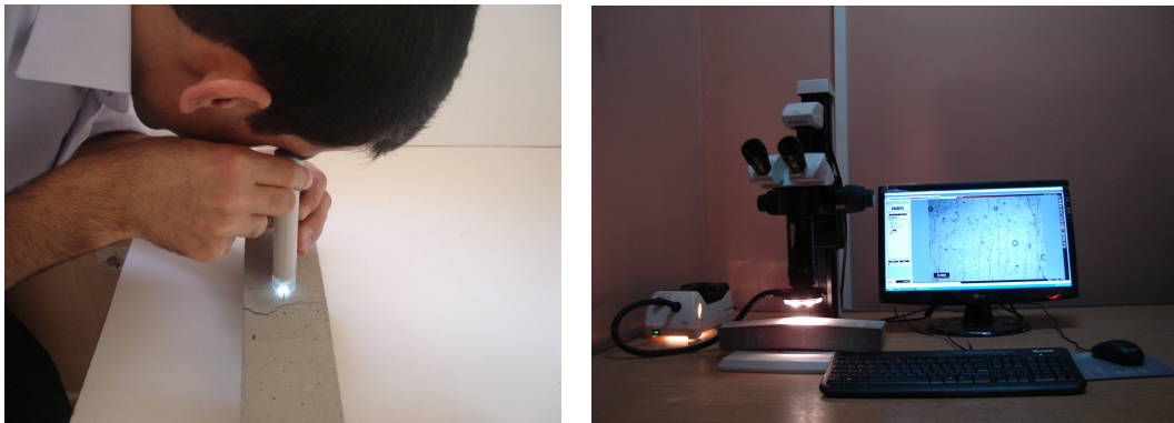
Figure 3.12. Control of crack widths of specimens tested by four-point test
