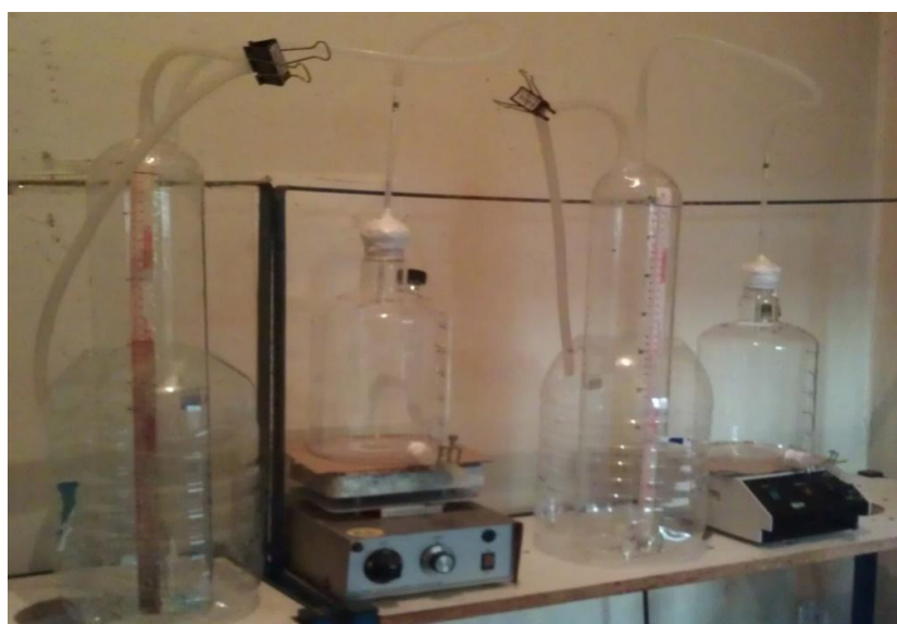
Figure 3-1: 2.5 liter anaerobic batch reactors
