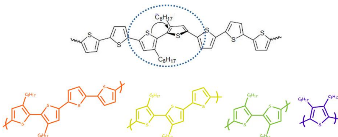
Figure 1.12 The interannular rotation of single bonds and resulted emission colors of conjugated polymers given in structure
