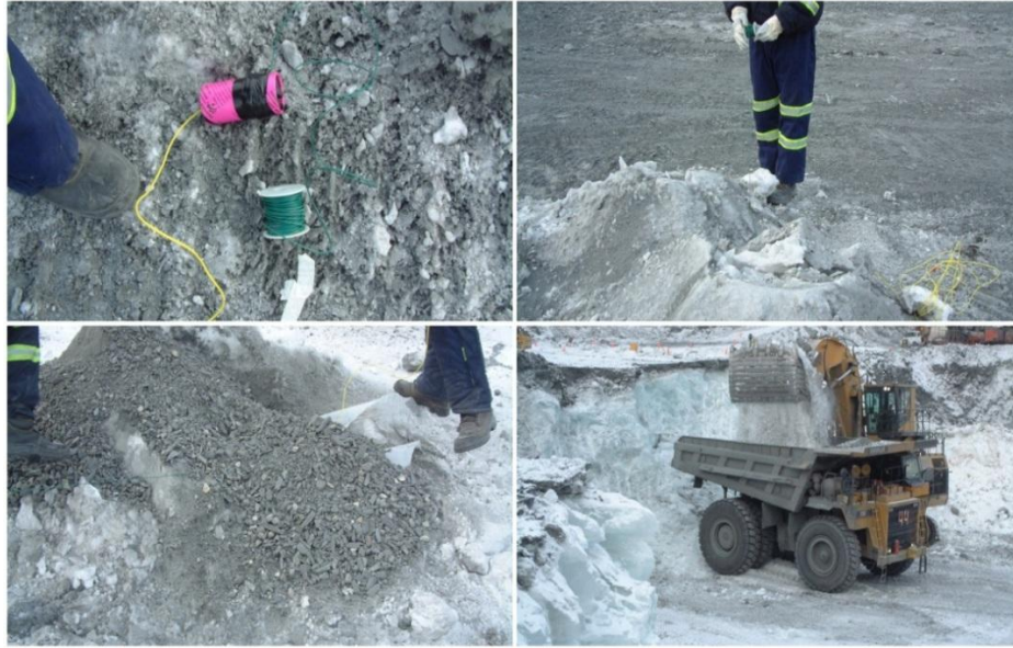
Figure 4.10 VOD measurements in glacier benches
